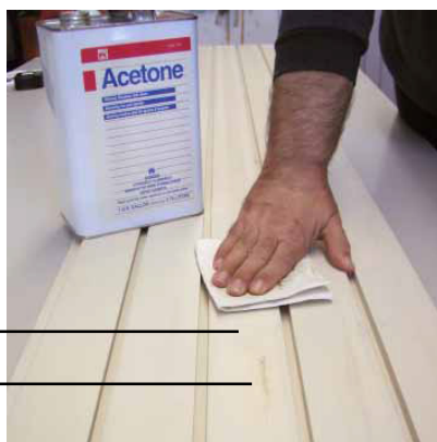
Scratches cleaned and removed
