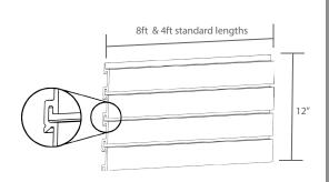
Patented backside slotted profile enables the use of SD InstallStrip for quick and easy installation
