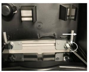
Step 5: Optional: Install the hose retainer on the front panel with the two small black screws. There is a small indentation on the retainer where the screws can pernitrate. Note that when installed you should be able to read the word "Warning".
